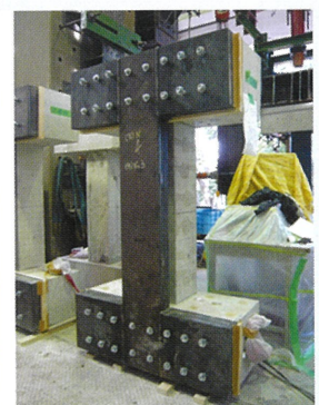
外付け鉄骨耐震補強 Seismic Retrofit Using Outer Steel Frame
